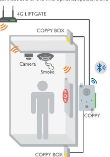
The button management on Coppy BOX is performed through **2 wires only** and no other connection is required.
