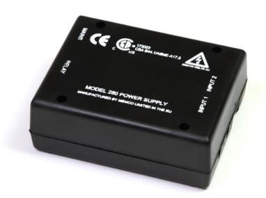
Memco 280 series power supply units (PSU) and control devices offer regulated 24VDC power supply for selected Memco light curtains. A range of input voltages are available to suit different requirements. The light curtain semiconductor output is converted to a potential-free relay contact providing greater control flexibility.
