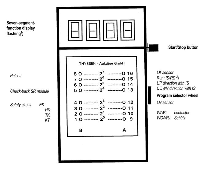
Altogether 16 functions can be interrogated or handled with diagnostic unit I. The individual functions can be set with the program selector wheel. The selected function appears in the seven-segment display (flashing display).
