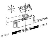
1 NO contact BN 310-10Z with N-S actuating magnet
