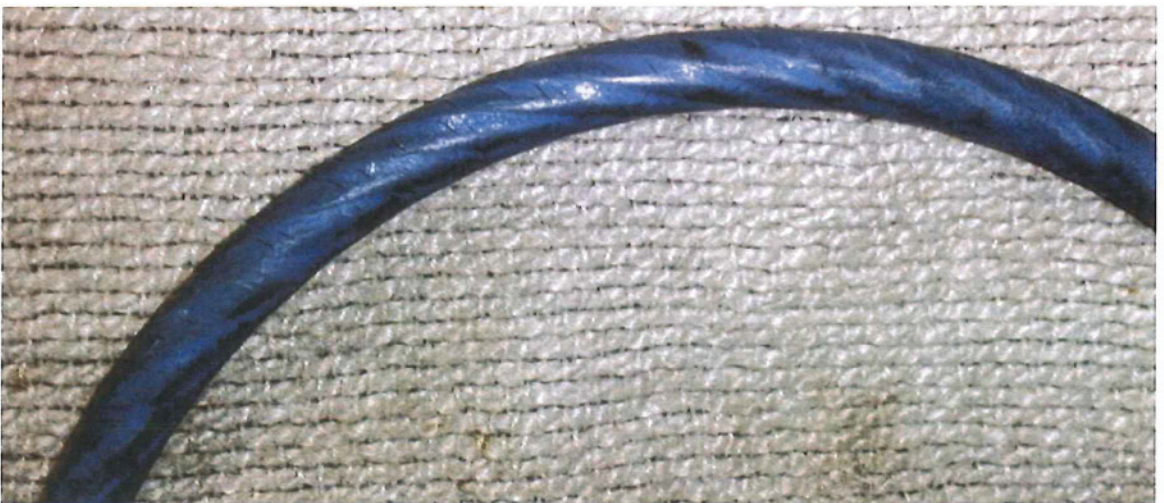
Fig. 2: Sheath tears on barely dirty rope section
