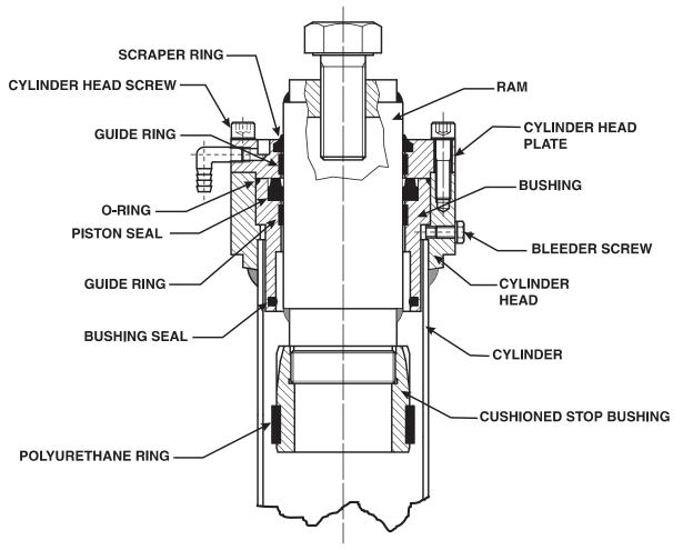
Secure the car in such a position that , by standing on the roof of it , you can check the ram which moves downwards and work on the cylinder head ; if the installation is a 2:1 instal lation , then take off the ropes.
